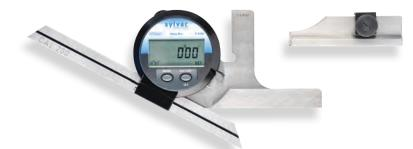
Fowler-Sylvac's Deluxe Electronic Protractor, featuring the patented Sylvac measuring system, provides an LCD readout in 1 minute of arc or 0.01 degrees of arc. A push-button selects the range according to application (1 x 360°, 2 x 180° or 4 x 90°) and changes the reading from arc minutes to decimal degrees. Additional push-buttons provide "reset" and "print" functions.
