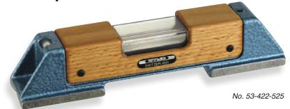
The Fowler-Wyler Horizontal Spirit Level is used for inspecting and levelling horizontal surfaces and cylinders. Sensitivity of .0005" per 10" length. This model features prismatic bearing surface, longitudinal and cross levels. Levels feature numerous advantages and ensure easy, accurate measurements.
