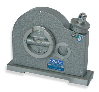
Use to set and check angles through 360°. Used in industries such as machine tools, general engineering, shipbuilding, textile machinery, structural bridges, mining & aeronautical, etc.
