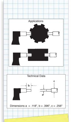
Measure recesses, grooves & splines
